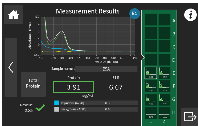
Figure 4: Illustration of the Results screen on the Little Lunatic. Unmix app results of the selected sample are shown as spectral shape as well as in calculated values.
