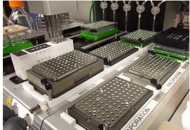
Heated filter block on temperature controlled station
